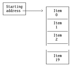
The starting address of an array declared as "real" is handled as a real variable even though it contains a 32-bit address pointing to its data. The address is in the first four of the eight bytes (low byte first).
