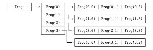
Like the variable Frog, the elements Frog(0) through Frog(3) contain addresses that point to arrays. These arrays are the second dimension of the original array, Frog.
