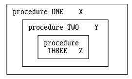
The statements inside procedure ONE can call procedure TWO because both the call and procedure TWO are within procedure ONE. However, the statements inside procedure ONE cannot call procedure THREE because the scope of THREE ends at the end of procedure TWO.
